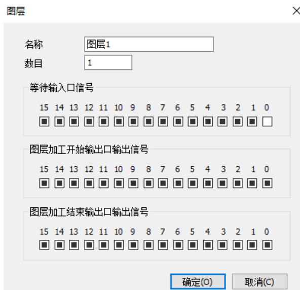
Figure 7.3 Setting Layer Corresponding Switches
